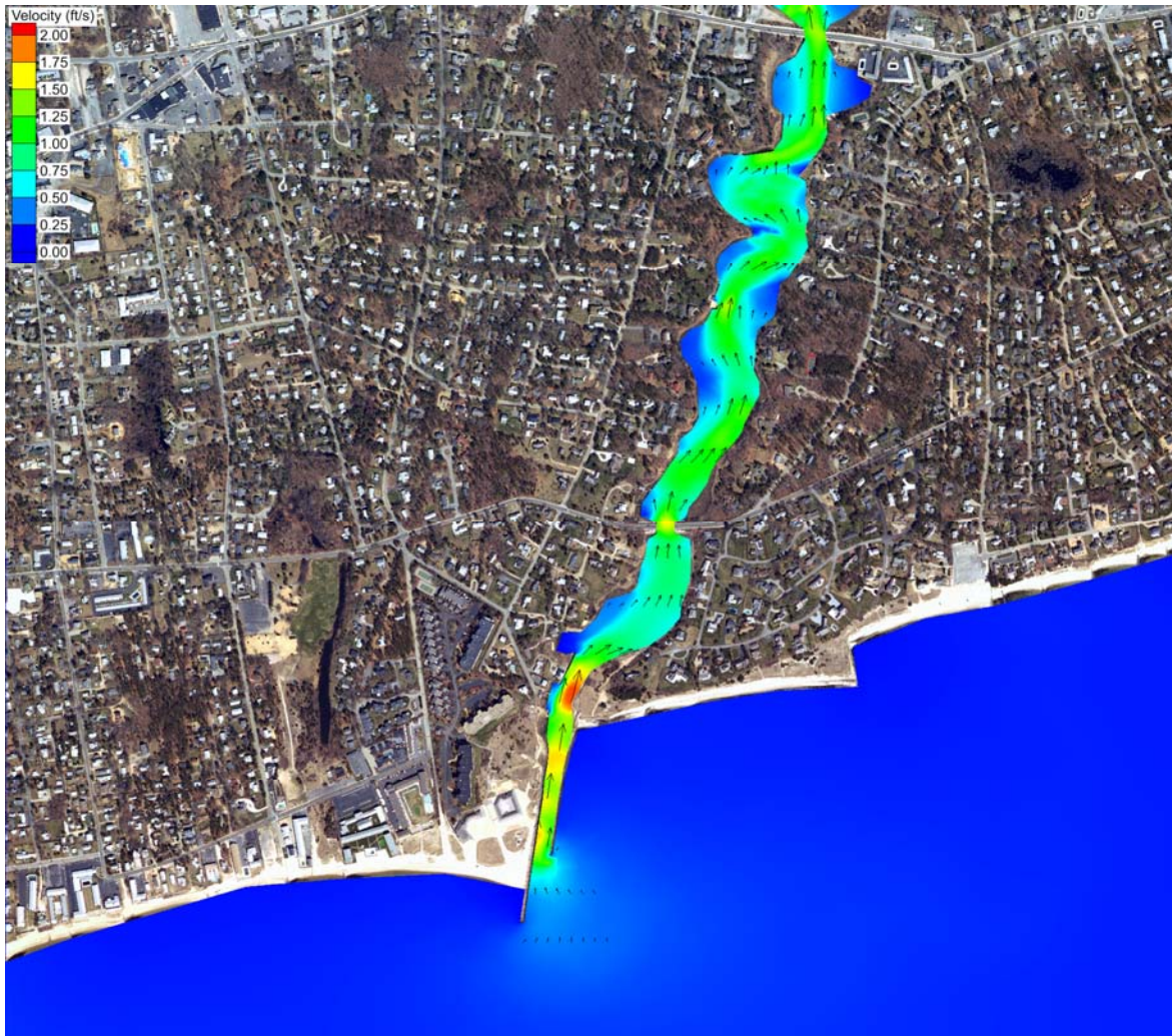
Figure V-17. Example of hydrodynamic model output for a single time step where maximum flood velocities occur for this tide cycle. Color contours indicate velocity magnitude, and vectors indicate the direction of flow.
