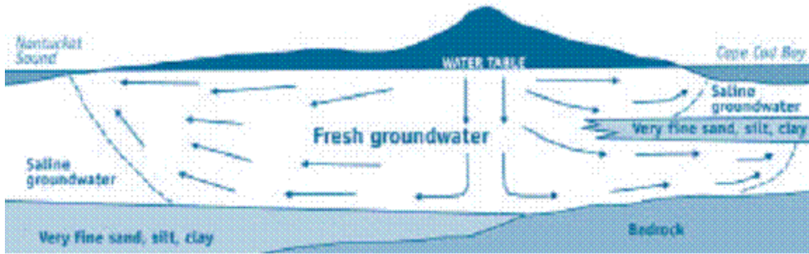
Figure 6: Hydrogeologic cross-section of the Monomoy Groundwater Lens modified from USGS Hydrologic Atlas HA-692, 1986 (vertical exaggeration x10).
