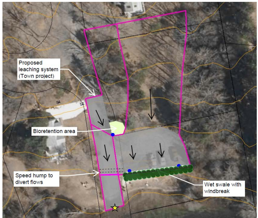
Site Sketch: Drainage area in pink, impervious cover in gray, BMPs in light green, revegetation in dark green, and proposed paved flumes in dark blue. Star represents the GIS location of the boat ramp.
