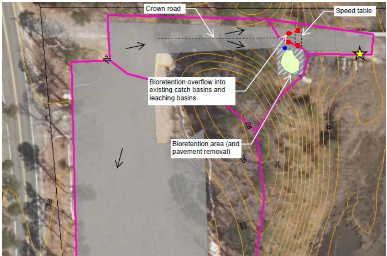
Site Sketch: Drainage area (pink), impervious cover (gray), impervious cover reduction (striped gray), BMPs (light green), paved flumes (dark blue), existing infrastructure (red), and drainage flow paths (arrows). Star represents the GIS location of the boat ramp.
