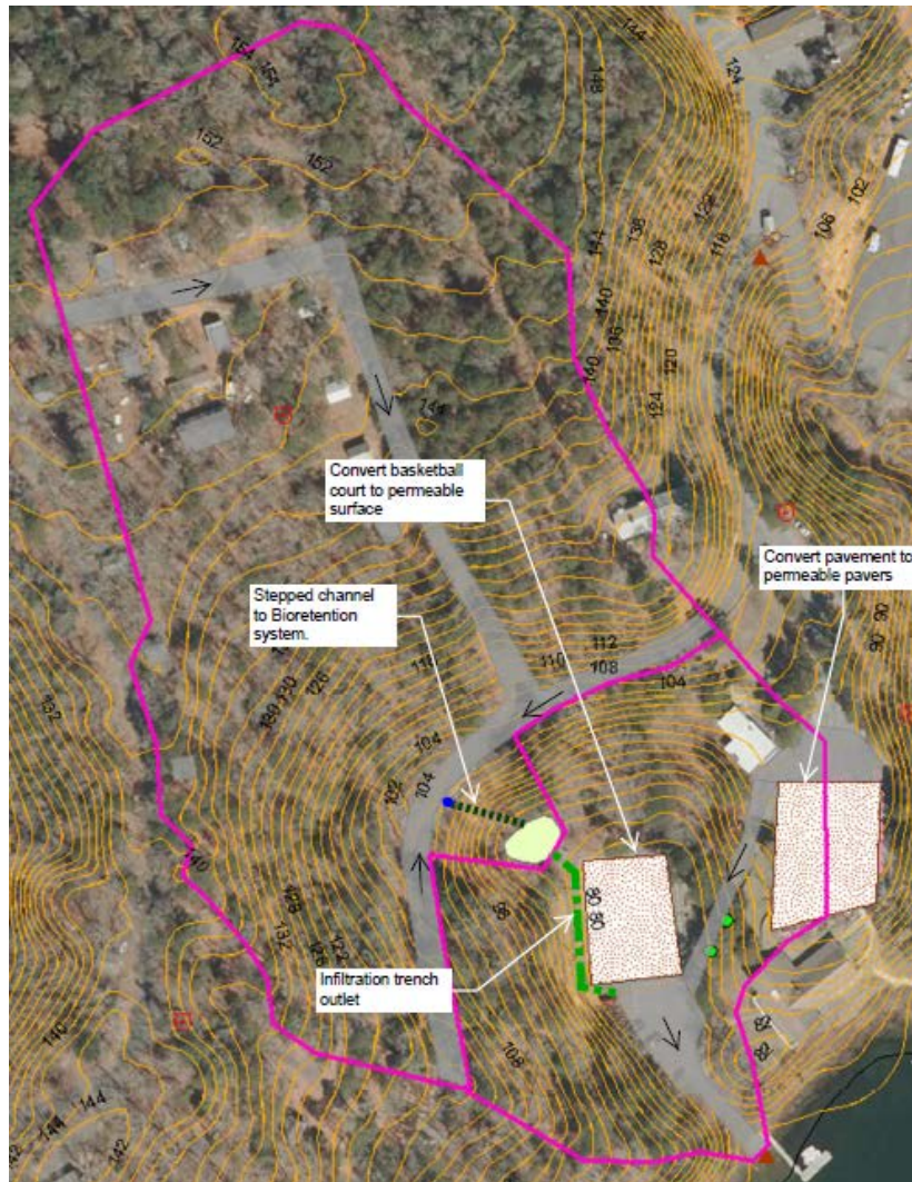
Site Sketch: Drainage area (pink), impervious cover (gray), BMPs (light/dark green and speckled brown), paved flumes (dark blue), existing outfalls (green circles), and drainage flow paths (arrows). Star represents the GIS location of the boat ramp.
