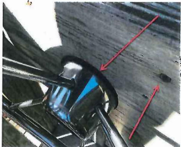
HARDWARE IS LOOSE AND BACKING OUT BY THE WHEEL. THIS IS PINCH & CRUSH POINT HAZARD.
