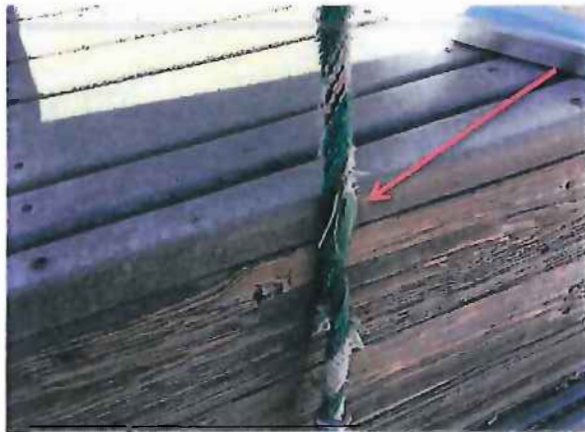
INCREASED WEAR FROM 2018 AUDIT. MORE STEEL STRANDS ARE EXPOSED.
