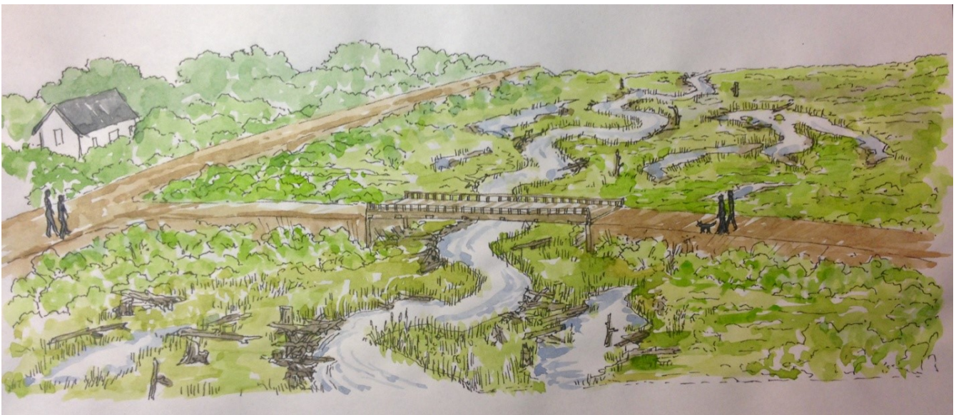
Figure 2: An example of a rendering of a retired cranberry bog that has been ecologically restored with habitat details including large wood to provide habitat for a variety of wildlife, channel bed geometry, micro-topography, recreational opportunities, and natural vegetation. (source: Nick Nelson, Inter-Fluve)
