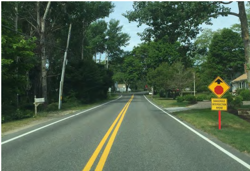
Figure 8 – Pleasant Bay Road westbound approach showing partially obscured stop sign
