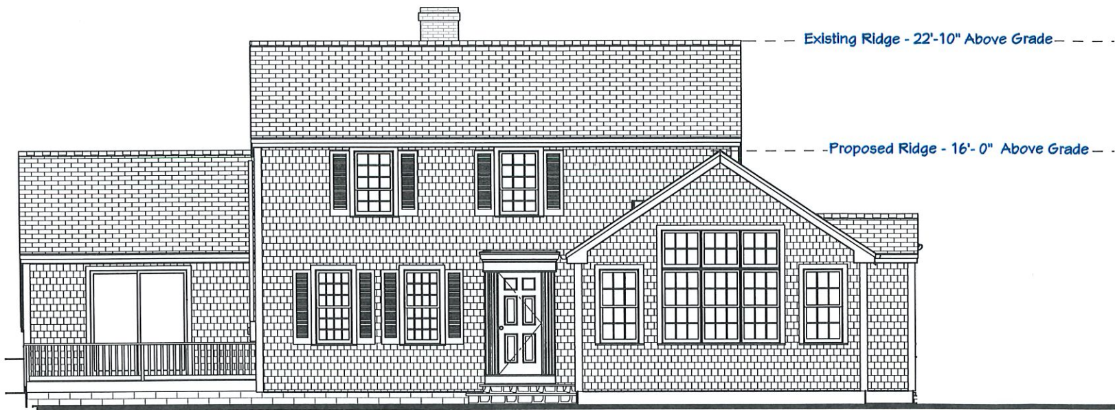
Exterior Elevation Front 1/8 in = 1 ft Marcille - 1.2
