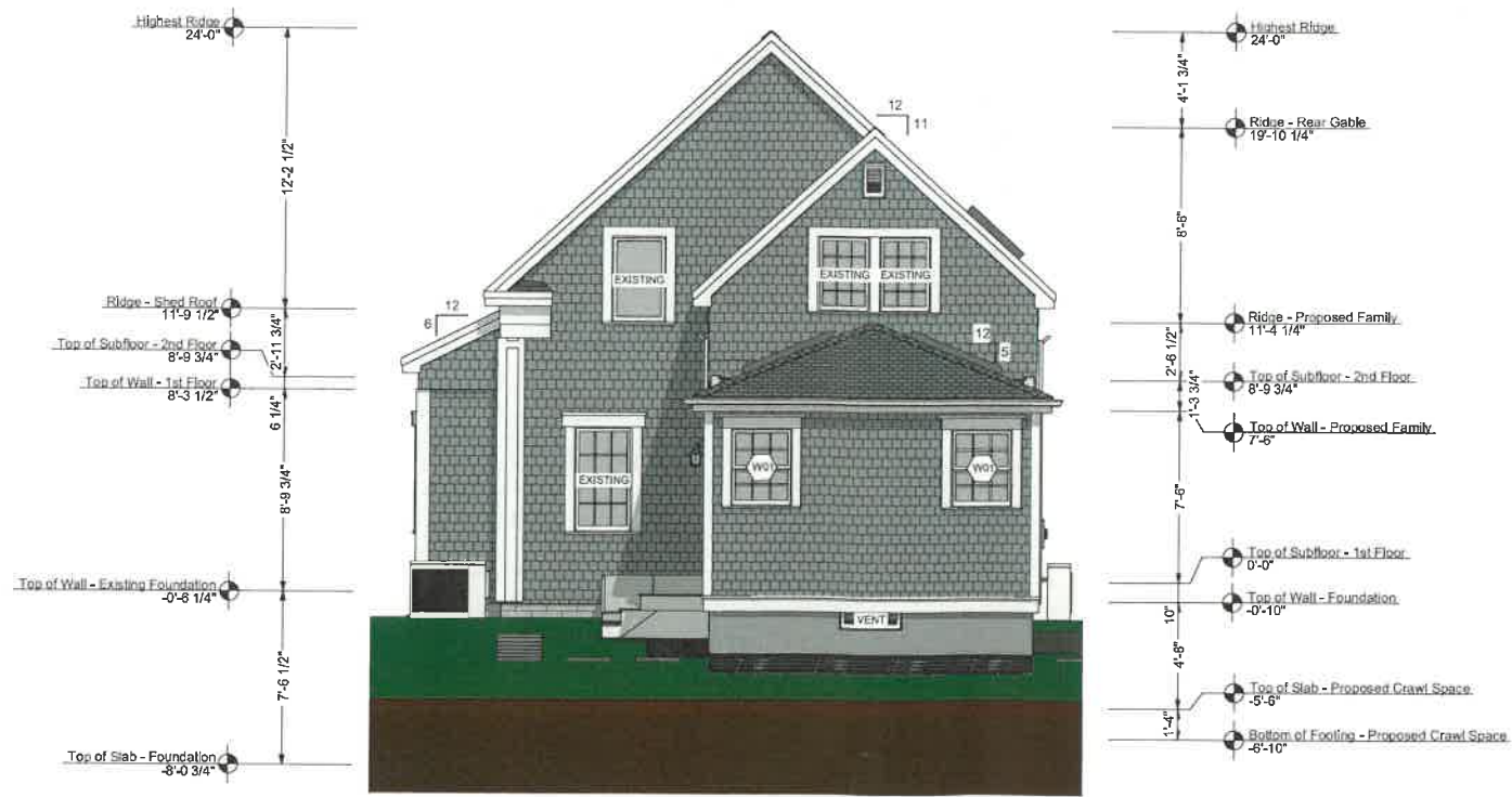
B PROPOSED REAR ELEVATION A2.3 SCALE: 1/4" = 1'-0"
