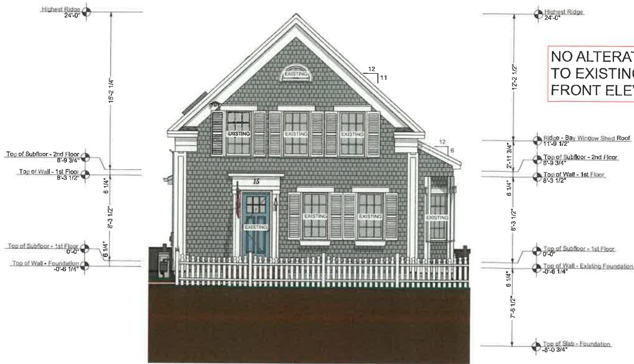
B PROPOSED FRONT ELEVATION A2.1 SCALE: 1/4" = 1'-0"
