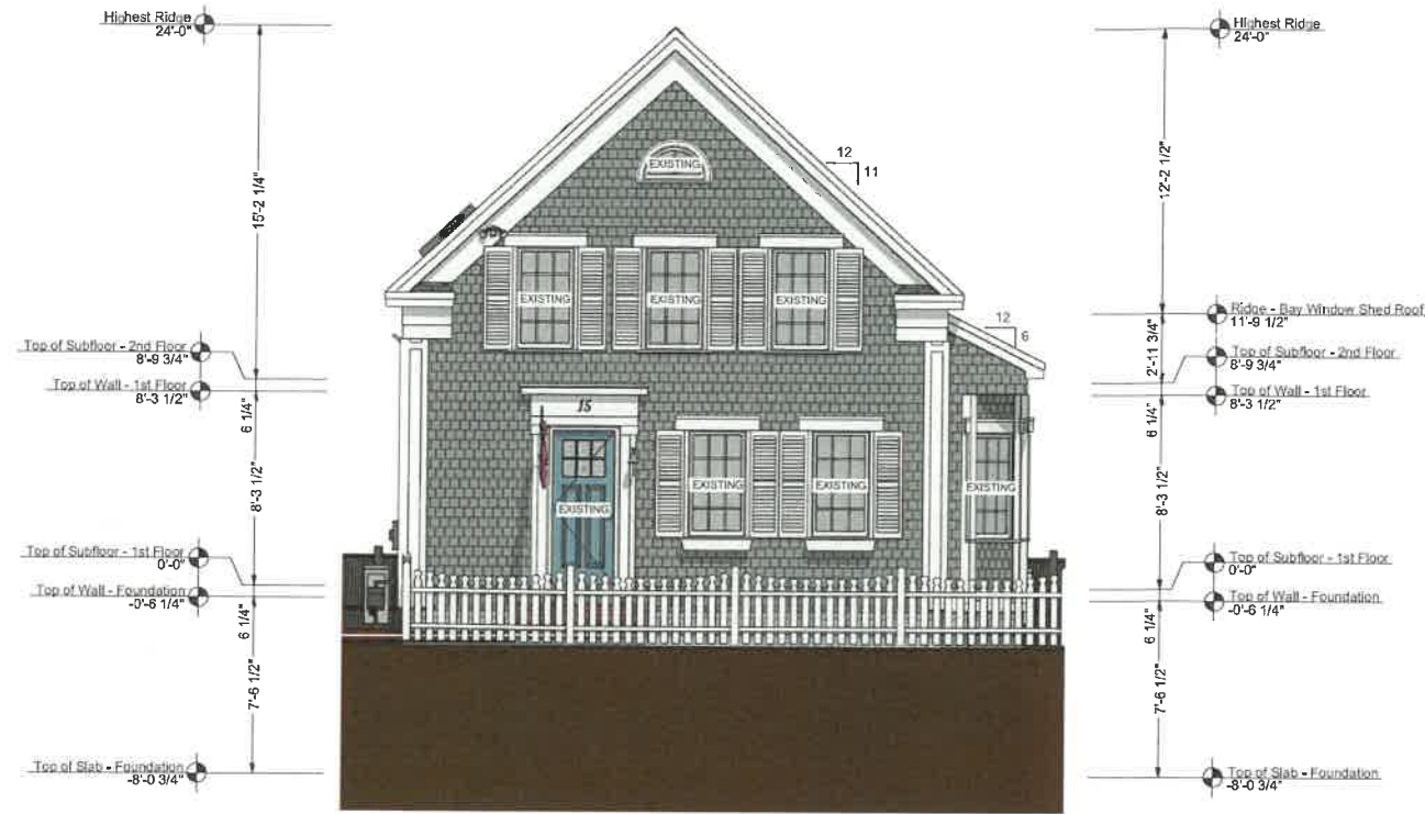
A EXISTING FRONT ELEVATION A2.1 SCALE: 1/4" = 1'-0"
