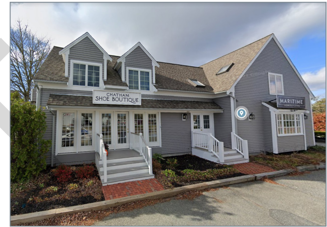
Stepbacks in the facade, multiple entries, and varied window patterns with vertical shapes help this building reflect traditional facade designs. Image: Google maps.
