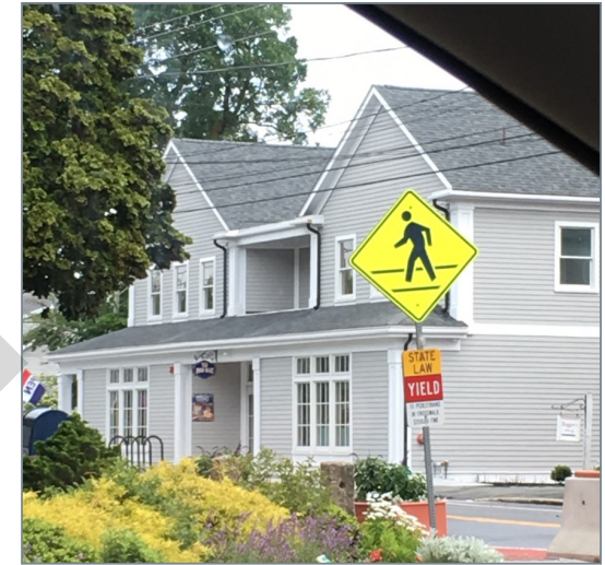
This new building incorporates narrow gable roof forms, a stepped back second floor, and street-facing display windows to continue historic building patterns.
